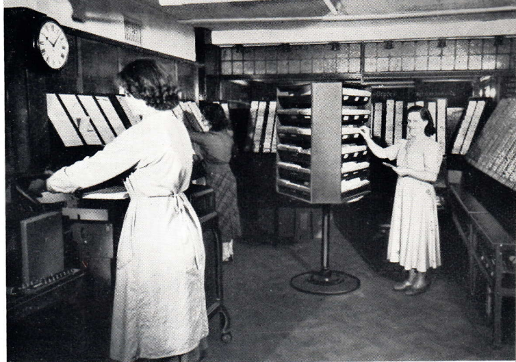
A view of the master pre-punched commodity card files. In the centre is a revolving file holding cards for all normal quantities of rationed goods.
